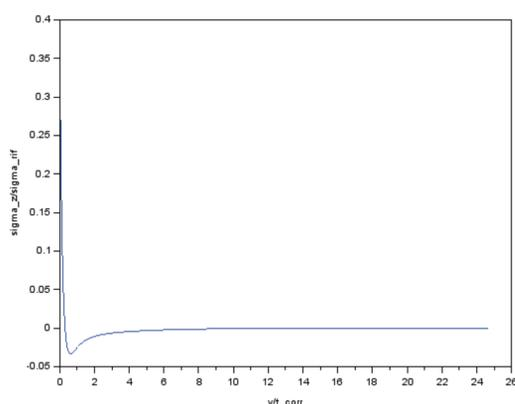
Setting a failure criteria, stresses distribution may describe an **incipient delamination/debonding**
