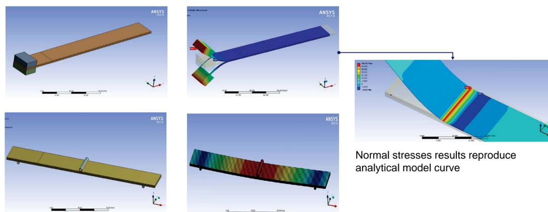
Second activity: Application of calibrated CZM to aeronautical composite-made structures with a **de-bond defect** (indicated with a red circle), in order to provide residual strain and fracture strength.
