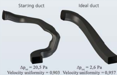
Duct geometry
