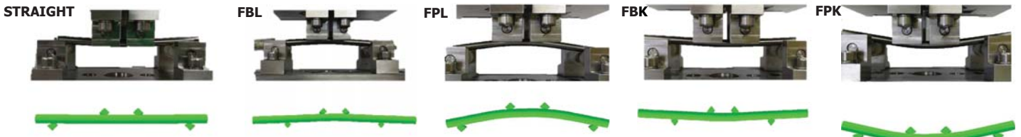
Figure 5: Summary of experimental and numerical fatigue testing configurations, regarding Straight rods (S), French bender (FB) and homogeneously bent rods through Four points bending (FP). The fatigue configurations are lordotic (L) and kyphotic (K).
