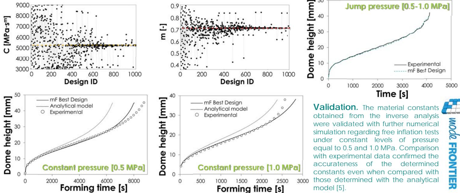
**Validation.** The material constants obtained from the inverse analysis were validated with further numerical simulation regarding free inflation tests under constant levels of pressure equal to 0.5 and 1.0 MPa. Comparison with experimental data confirmed the accurateness of the determined constants even when compared with those determined with the analytical model [5].
