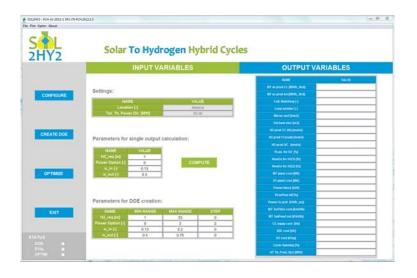
EnginSoft developed a new software tool to make a flexible plant design with different share of cycle opening, SO2 source, solar energy share and, on demand, adjustable hydrogen production. Namely, it is capable to estimate CAPEX/OPEX for any planned location.
