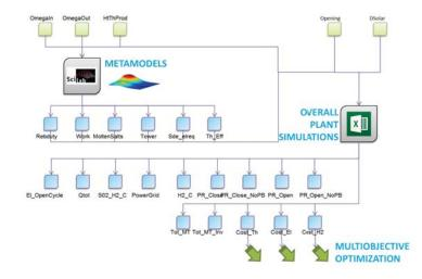
The creation of the optimization process of the whole plant brought also to the development of a platform that integrates the simulation spreadsheets and metamodeling techniques, which are also useful to deal with the size (scaling) of the solar plant under consideration.
