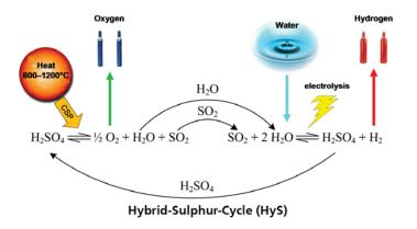
The project aims to develop and demonstrate all key components of the HySprocess - solar sulphuric acid cracker, sulphur dioxide depolarized electrolysis, gas separation, heat storage - at industrial relevant scale.
