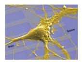
Establishing a reliable communication with real neurons through ad-hoc developed electronic transducers for recording and stimulation of electrical activity.
